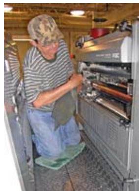
Part of the press is moved into place, top photo. Above, press operator Keith Young cleans it. Before leaving the factory, the press is encased in a waxy protective coating, called Cosmoline®, to prevent salt water from corroding it on its overseas voyage. Young must clean every surface, nook, and cranny for the press to work properly.
