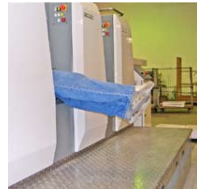
Part of the press is moved into place, top photo. Above, press operator Keith Young cleans it. Before leaving the factory, the press is encased in a waxy protective coating, called Cosmoline®, to prevent salt water from corroding it on its overseas voyage. Young must clean every surface, nook, and cranny for the press to work properly.
