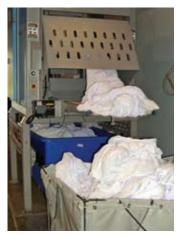
The metal arm of the Pik-Quik (behind the bar at the front of the machine) reaches into a tangle of clean sheets in the blue bin to pull one up and shake it loose. The arm will then feed the sheet onto rollers that will push it out into the pile of untangled sheets in the gray bin.
